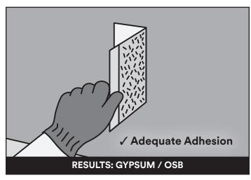
If the  $3M^{\mathbb{M}}$  Air and Vapor Barrier 3015NP test strip is stuck to exterior gypsum or OSB, you should notice small fibers pulling from the substrate. If you are seeing these results, you can be confident you have adequate initial adhesion to continue applying to the walls.
