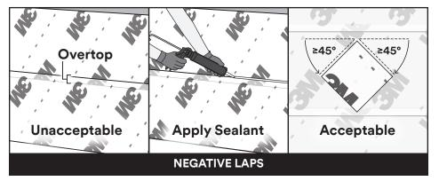
On a vertical surface with multiple horizontal rows of tape, negative laps are created when the **lower tape is applied overtop** of the higher tape. To address a negative lap, apply a bead of 3M<sup>™</sup> Polyurethane Adhesive Sealant 540 or 3M<sup>™</sup> Adhesive Sealant 740 UV (or equivalent) to the seam. For any negative lap where the covering tape is applied at a **45° or greater angle** from a horizontal tape, no sealant is needed.
