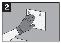
Stick the test strip to the substrate you intend to cover and apply pressure.
