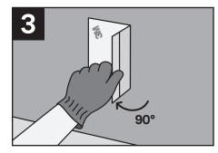
Slowly remove the test strip, pulling the tab up at approximately a 90° angle.
