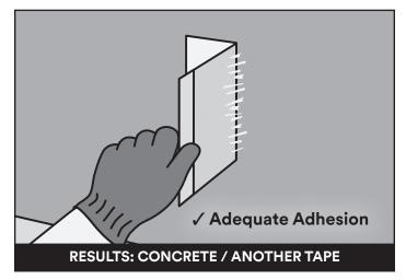
If the  $3M^{\sim}$  Air and Vapor Barrier 3015NP test strip is adhered to concrete or another tape, you should see small "legs" where the adhesive is stretching between the tape backing and the substrate. If you are seeing these results, you can be confident you have adequate initial adhesion to continue applying to the walls.
