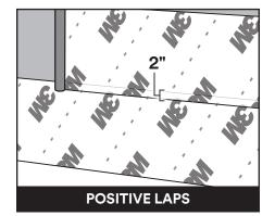
On a vertical surface with multiple horizontal rows of tape, positive laps are created when the **higher tape covers the tape below it**.
