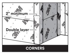
Inside/outside corners should have a double layer of 3M<sup>™</sup> Air and Vapor Barrier 3015NP and will require at least a 6" wide piece to ensure there is a 2" minimum double layer on the entire corner.
