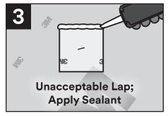
If the patch is applied at less than a  $45^{\circ}$  angle, the top edge will need a bead of sealant.
