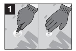
Poke or make a small slit to pop the bubble. Force the entrapped air out.
