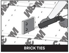
Brick tie detailing requires a minimum of 2" tape on all sides, along with a bead of sealant around the entire brick tie. It is acceptable to apply the sealant before or after the tape is applied.
