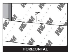
Horizontal wall applications require a 2" minimum overlap. Start application at the bottom and work upwards to create positive laps.
