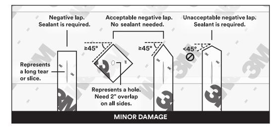
Small holes or damaged areas of the tape can easily be repaired with 3M<sup>™</sup> Air and Vapor Barrier 3015NP. Follow the same negative/positive lap guidelines for repairing damaged areas. If damage affects the surface beneath the tape, holes 1/4"-1/2" require sealant and holes greater than 1/2" require a backer rod and sealant.
