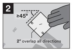
Apply a patch of 3M<sup>™</sup> Air and Vapor Barrier 3015NP over the hole at a 45° angle to create an acceptable negative lap. Ensure a 2" minimum overlap in all directions.
