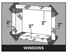
Window detailing requires a 2" minimum overlap with the field tape.
