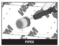
Pipe penetrations should be flashed with 3M<sup>™</sup> Ultra Conformable Flashing Tape 3015UC with a minimum of 2" on the wall and 2" on the pipe. A bead of sealant should be applied to the top of where the field tape and the 3M<sup>™</sup> Ultra Conformable Flashing Tape 3015UC meet.
