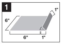
Cut approximately a 6" x 8" piece of  $3M^{\mathbb{W}}$  Air and Vapor Barrier 3015NP tape. On the adhesive side fold 1" over onto itself to create a 6" x 6" test strip with a finger tab.
