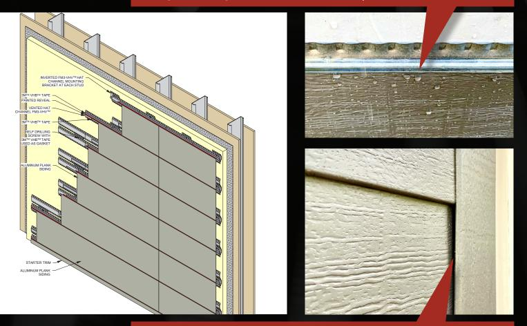
VentClad<sup>™</sup> "Stick-On" Trim with 3M<sup>™</sup> VHB<sup>™</sup> tape makes installation quick & easy while ELIMINATING fasteners
